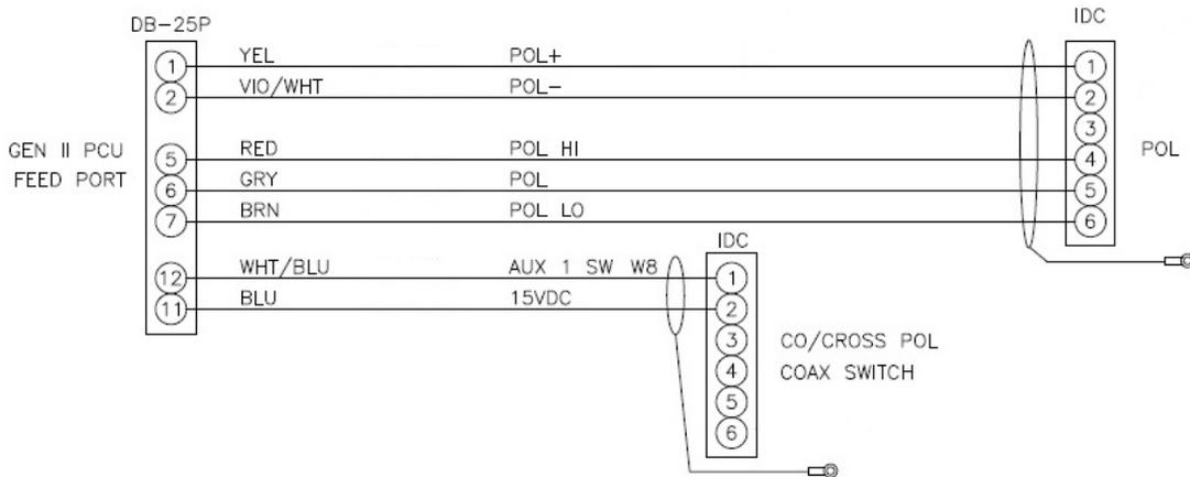
If the harness connections are good, then the PCU motherboard isn't outputting the voltage to drive the motor and needs replacing.
