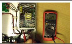
2. Now measure the output voltage from the power supply on the connectors for the red (+) and black (-) cables on the right of the connection block, the output should be 24VDC.
