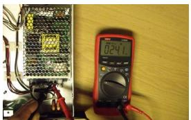
If the units AC input has been verified and the 24VDC is not present, the power supply is defective and needs to be replaced. If the power supply is outputting the 24VDC consistently then the power supply is operational and the problem lies elsewhere (possible failure with the PCU, DAC motherboard or harness connection).
