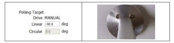
The feed horn should rotate 45.0 degrees clockwise (when viewed from the front of the reflector) so that the alignment marks of the phase card in the feed horn are aligned vertically, from left to right (as shown above).
