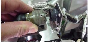
3. Remove the 5 screws which securing the mounting plate with the cannon connection and IDC connection PCB to the RF cage. Retain the hardware for future use.
