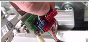
30. Secure the pot, motor and sensor harness to the underside of the upper bracket using a cable tie.
