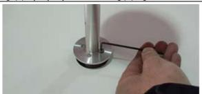
2. Disconnect the military spec connector from its socket to allow access to the screws to remove the upper bracket.
