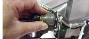
33. Reinstall the feed horn using the hardware removed in step 1, tighten with a 2.5mm Allen wrench. Apply Loctite 242 to the threads.
