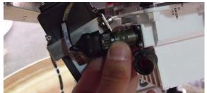
29. Sit the upper bracket on top of the RF cage and reconnect the IDC connectors with the 4-pin sensor connector on the left, the 5-pin pot connector in the center and the 2-pin motor connector on the right (as shown in the image on the right).
