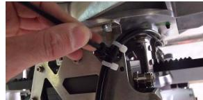
28. Route the BUC DC power cable around between X-Pol LNB and the RF cage and connect it to the BUC.
