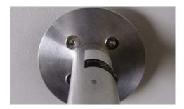
Any error in alignment is an indication that the pol pot is not correctly calibrated. However a small amount of error could be calibrated out by using the linear offset setting (to electronically adjust the pol postion).
