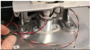
18. Remove the cable wrap to free the pol pot harness so the assembly can be removed.
