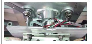
14. Using a 3mm Allen wrench remove the 4 screws from the waveguide flange mated to the Co-Pol LNB. Save the hardware for future use.
