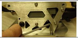
16. Remove the bracket along with the Co-Pol LNB as a complete assembly to allow access to the pol pot assembly.
