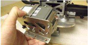
17. Using a 3mm Allen wrench loosed the pol motor screws enough to allow the backlash gear to be disengaged from the main sprocket.
