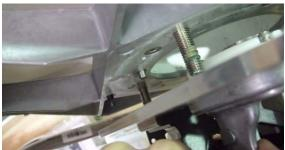
39. Using the hardware removed in step 12 secure the RF cage to the rear of the reflector using a 17mm wrench. Apply Loctite 242 to the threads.
