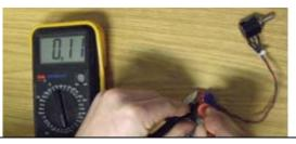
Leaving the pot at its counter clockwise end stop measure between the clockwise contact and the slider (grey cable, pin 2 on the IDC connector and the brown cable pin 1 on the IDC connector) the resistance should be reversed from the previous rotation, reading 5 ohms. Rotating the shaft of the pot clockwise should reduce the resistance through its range to 0 ohms. Any error with the pot not giving the correct resistance is an indication the pot is defective and needs replacing.
