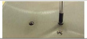
4. Remove the 3 screws securing the power supply to its mounting bracket using a #1 Phillips screwdriver. Save the hardware for future use.
