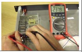
2. Now measure the output voltage from the power supply on the connectors for the red (+) and black (-) cables on the right of the connection block, the output should be 24VDC.
