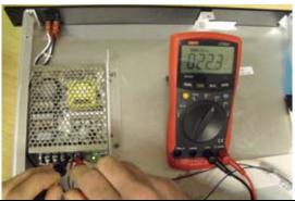
If the units AC input has been verified and the 24VDC is not present, the power supply is defective and needs to be replaced. If the power supply is outputting the 24VDC consistently then the power supply is operational and the problem lies elsewhere (possible failure with the MXP motherboard or harness connection).
