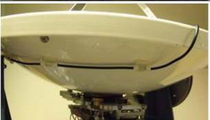
8. Apply loctite 242 to the thread and install the P-clip and retaining screw to the yoke, securing the GPS antenna harness. Rotate the reflector backwards and forwards ensuring there is enough slack on the harness and secure it by installing cable ties on either side of the P-clips.
