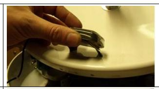
6. Install the 3M adhesive provided in the kit to the replacement GPS antenna and attach it to the reflector in the same position the defective one was removed from.
