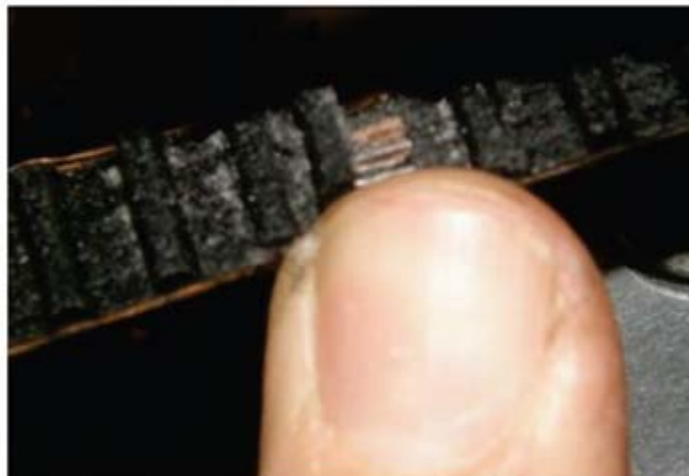
Seperating tooth and edge wear
