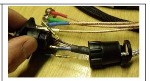
17. Screw the lower section of the harness onto the socket connector and attach the retainer using a #1 Phillips screwdriver.
