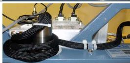
26. Feed the excess harness and connectors through the yoke of the system and connect the interface harness D-sub connector to the PCU using a 2mm flat blade screwdriver.
