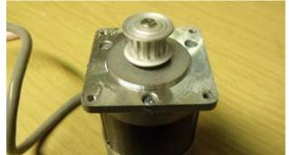
6. Apply Loctite 242 to the hardware removed in step 4 and loosely install the replacement azimuth motor assembly, slotting the motor pulley into the azimuth belt.
