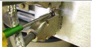
2. Cut the cable ties securing the azimuth motor harness using a pair of cutters.
