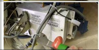
3. Now using an 8mm wrench back of the tensioning screw on the underside of the motor bracket to allow the motor to be removed.
