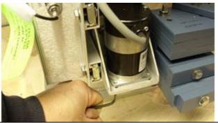
7. Ensure the belt is correctly installed over the motor pulley and in between the tensioning wheels and tighten the belt tensioning screw using an 8mm wrench.
