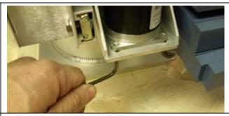
5. Apply Loctite 638 to the shaft of the replacement motor and fit the pulley in the same position as the one on the defective motor. Fit the set screw into the pulley with Loctite 222 using a 1/16" Allen wrench.
