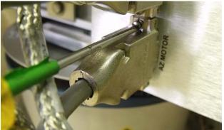
11. Secure the azimuth motor harness using cable ties.
