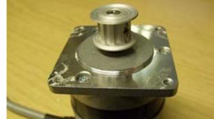
6. Apply Loctite 242 to the hardware removed in step 3 and install the replacement motor assembly, with the cable pointing downwards. For the 4<sup>th</sup> screw apply the Loctite to the thread of the motor.
