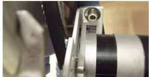
7. Using your hand apply pressure to the motor to tension the elevation belt and tighten two of the retaining screws.
