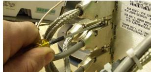
10. Secure the elevation motor harness using cable ties.
