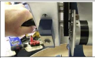
5. In the same orientation as on the defective motor install the new pulley to the replacement motor, applying Loctite 638 to the shaft. Apply Loctite 222 to the set screw and install it into the pulley, making sure it's aligned with the flat edge of the motor shaft. Tighten the set screw with a 1/16" Allen wrench.
