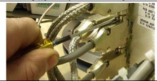
2. Cut the cable ties securing the elevation motor harness using a pair of cutters.
