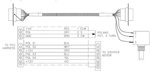
Check the harness for good continuity from point-to-point and that there are no shorts from wire-to-wire or from wire-to-ground that are not supposed to be there as per the above diagram. Repair any harness problems found and re-run the BIT tests. If there are no problems with any of the steps above, replace the PCU and re-run the BIT tests.
