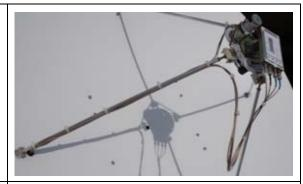
21. Secure excess harness behind the reflector and secure it under the elevation pan with a p-clip, applying Loctite 242 to the screw (as shown on the right).
