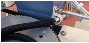
16. Using a 2mm flat blade screwdriver disconnect the interface harness D-sub connector from the PCU (lower right connector).
