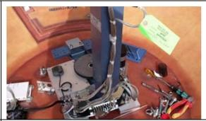
28. Secure the lower of the harness with cable ties allowing free movement of the base section (as shown on the right).
