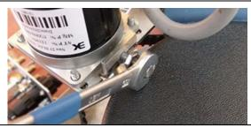
40. Slide the rear section of the harness socket connector over the harness.
