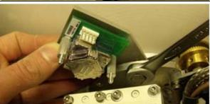
Connect the IDC connector to the rate sensor PCB. Ensure the harness isn't pulled taught, if so adjust the pivot position or the PCB mounting bracket.
