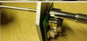
Install the sensor and bracket assembly to the feed using a 7/16" wrench, applying Loctite 2760 to the thread of the bolt.
