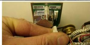
Remove the bracket from the feed using a 7/16" wrench. Save the hardware for future use.
