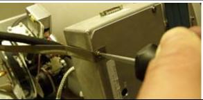
8. Connect the motion platform PCB D-sub connector to the elevation pan using a 2mm flat blade screwdriver.
