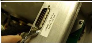
3. Remove the 6 screws securing the elevation pan cover to the using a #1 Phillips screwdriver. Save the hardware for future use.
