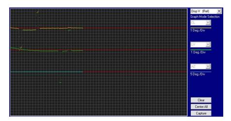
If using DacRemP the elevation trace should look similar to this image, note how after each movement the system returns to its level position efficiently without taking time to settle. Should the system take time to settle, or not stabilize to the original position (not necessarily on the red line) then this is an indication that the antenna isn't maintaining its horizon reference correctly and further troubleshooting will need to be undertaken.
