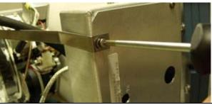
4. Remove the 3 screws securing the defective motion platform PCB to the elevation pan using a #1 Phillips screwdriver. Remove the defective motion platform PCB, save the hardware for future use.
