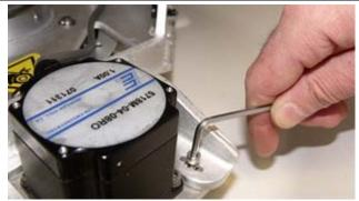
8. Apply Loctite 242 to the thread of the tensioning screw and tighten it using a 10mm wrench. Periodically check the belt tension as per the following step.
