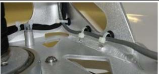
13. Refit the PCU PCB cover using the hardware removed in step 1. Apply Loctite 242 to the threads.
