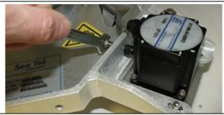
5. Undo the four screws mounting the azimuth motor assembly to the yoke. Save the hardware for future use.
