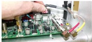
3. Using a pair of cutters snip the cable ties securing the azimuth motor harness to the yoke.
