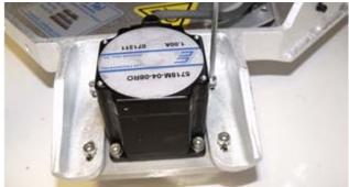
6. Install the replacement motor assembly by slipping the pulley through the belt ensuring it's correctly installed on the tensioning wheel (located under the yoke and in front of the motor mounting point).
