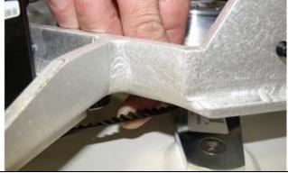
12. Secure the azimuth motor harness to the yoke, using cable ties.
