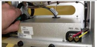
2. Disconnect the azimuth motor IDC connector from PCU PCB.
