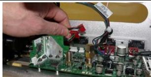
3. Cut the cable ties securing the elevation motor and encoder harnesses to the yoke using a pair of snips.
