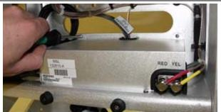
2. Disconnect the elevation motor and encoder IDC connectors from the PCU PCB.
