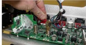
11. Secure the elevation motor and encoder harnesses to the yoke using a cable tie.
