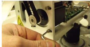
6. Install the replacement motor assembly with the harness pointing to the rear or the pedestal. Apply Loctite 242 to the threads of the hardware removed in the previous step. Do not fully tighten them at this time.
