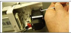
11. Secure the pol motor, encoder and coax cables, with the P-clip removed in step 4 and install the securing nut and washer. Apply Loctite 242 to the thread.
