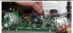
13. Secure the pol motor, encoder harnesses and coax cables with cable ties.
