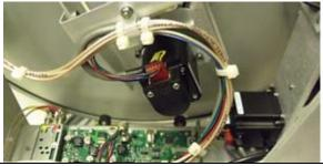
14. Install the PCU cover using the four screws removed in step one, apply Loctite 242 to the threads.
