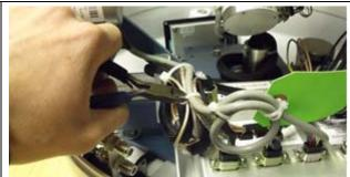
2. Disconnect the elevation motor D-sub connector from the PCU using a #1 Phillips screwdriver. Save the hardware for future use.
