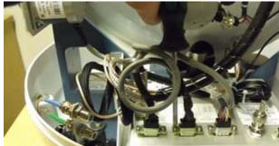
3. Using a #1 Phillips screwdriver remove the 4 screws securing the elevation motor to its bracket. The pulley will have to be rotated to allow access to the upper left screw (as shown on the right). Save the hardware for future use.
