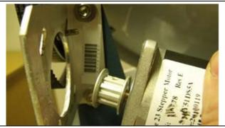
5. Install the replacement pulley onto the motor shaft in the same position as on the defective motor. Apply Loctite 638 to the shaft of the motor and install the set screw with Loctite 222 making sure it's against the flat edge of the motor shaft, tighten with a 1/16" Allen wrench.
