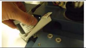
6. Remove the 4 screws securing the motor to the bracket using a #1 Phillips screwdriver, save the hardware for future use.
