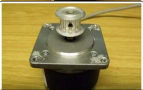
8. Apply Loctite 242 to the four screws and install the bracket to the replacement motor assembly with the harness cable exiting towards the mounting points (as shown on the right).
