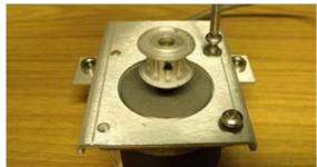
7. Install the replacement pulley onto the motor shaft in the same position as on the defective motor. Apply Loctite 638 to the shaft of the motor and install the set screw with Loctite 222 making sure it's against the flat edge of the motor shaft, tighten with a 1/16" Allen wrench.
