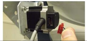
${\tt 3}.$  Snip the cable ties securing the elevation motor and encoder harness.
