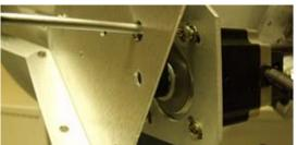
6. Install the pulley to the replacement motor in the same position as on the defective motor. Apply Loctite 638 to the shaft of the motor and install the set screw with Loctite 222 using a 1/16" Allen wrench. Ensure the set screw is installed against the flat edge of the motor shaft. Save the hardware for future use.
