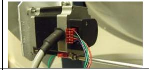
2. Disconnect the IDC connector from the encoder on the elevation motor.
