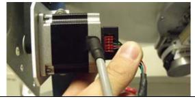
11. Reconnect the elevation motor harness to the PCU, ensuring the split washers are installed (no need to Loctite).
