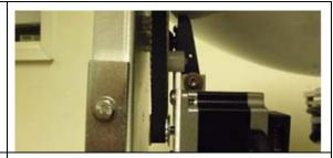
10. Reinstall the encoder harness and ground connection to the motor assembly using the hardware removed in step 1.
