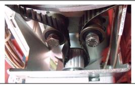
10. Support the motor and pull the belt over the top of the cross level sprocket, then rotate the cross level axis from left to right and work the belt onto the main sprocket.
