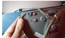
11. Apply Loctite 242 to the four screws and loosely install the cross level motor assembly.
