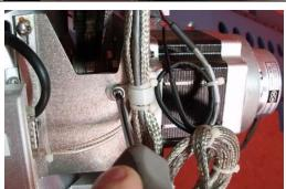
3. Remove the cable ties securing the motor harness.
