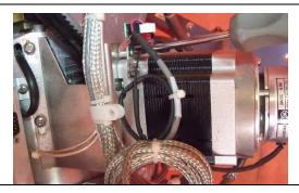
5. Disconnect the IDC connector for the cross level motor brake from the termination block (leave the main harness connected). Take care not to lose the hardware.
