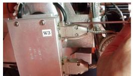
2. Undo the screw securing the P-clip and motor harness to the cross level motor bracket.
