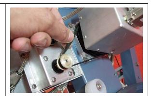
8. Reconnect the reference harness to the level cage motor assembly.
