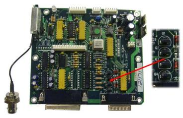
Set your multi-meter to the Diode setting and test between the pins of the transistors as per the following procedure and verify the results.
