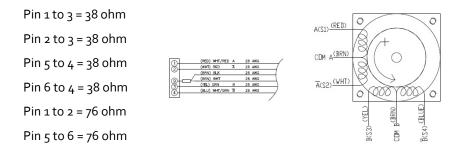
If one of the measuring points is open (no resistance) the motor is defective and need to be replaced. Also measure from all the pins to ground (the metal case of the motor) they must be open, not shorted.
