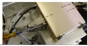
6. Using a ¼" wrench undo the standoffs to remove the modem.
