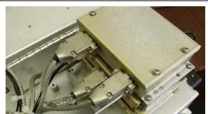
2. Now using a #1 Phillips screwdriver remove the 4 screws securing the pol aux relay to the assembly and remove it.
