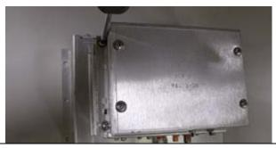
9. Disconnect the SMA cable from the upper MUX using a 5/32" wrench.
