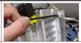
16. Reconnect the AC lead to the power supply and secure it in place with a cable tie.
