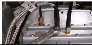
19. Install the remaining 2 screws to the mounts at the top of the polang relay with Loctite 222, securing the pclips and harness to the assembly.
