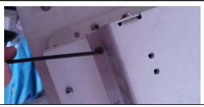
5. Apply Loctite 242 to the 4 screws removed earlier & install the replacement power supply.
