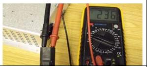
Now measure the output voltage from the power supply, to the pedestal on connection J1. 24VDC should be present between pin 9 (+) and pin 5 (-).
