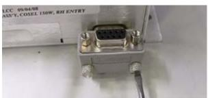
12. Install the MUXs onto the power supply, applying Loctite 222 to the standoffs.
