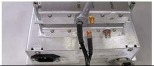
10. Remove the stand-offs securing the MUX(s) from the defective power supply using a 1/4" wrench.
