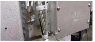
20. Install the pedestal DC D-sub connection to the 90 degree connector on the power supply assembly.
