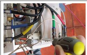
2. Remove the two upper screws securing the pol aux relay to the power supply.
