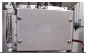
3. Reinstall the replacement pol relay applying Loctite 222 to the thread of the 4 screws.
