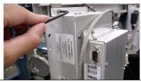
7. Using a #1 Phillips screwdriver remove the 4 screws securing the modem to the PCU.
