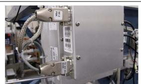
2. Undo the harness connections from the PCU using a 2mm flat blade screwdriver.
