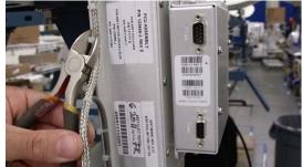
6. Using a 9/64" Allen wrench undo the 4 screws securing the PCU and modem assembly to the equipment frame.
