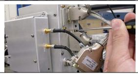
3. Undo the GPS antennas BNC connector from the PCU.
