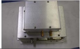
10. Re install the PCU to the equipment frame applying Loctite 242 to the threads. Ensure the mounting plates are correctly aligned on the rails of the equipment frame.
