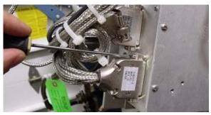
4. Using a 5/32" Allen wrench remove the 4 screws securing the PCU to the EL pan and remove the defective PCU assembly.
