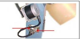
2. Using a 9/64" Allen wrench, remove the four Allen head screws securing the CL motor to its bracket and remove it.
