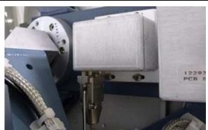
2. Undo the 4 retaining screws using a #1 Phillips screwdriver.
