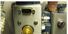
3. Install the replacement level cage motor assembly onto the pedestal. Install it low enabling the belt to be slipped over the pulley with no stress on it. Install the four screws and star washers loosely with loctite 242.
