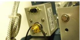
4. Tension the belt by sliding the motor assembly by hand away from the level cage and tighten <u>two</u> of the four screws.
