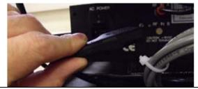
2. Disconnect the RX IN coax cable from the DAC.
