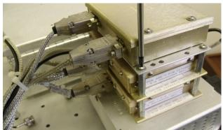
3. Using a 5/16" wrench undo the SMA cables from the modem, noting their orientation.
