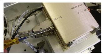
5. Using a ¼" wrench undo the standoffs to remove the modem (repeat the above procedures if the lower modem is to be replaced).
