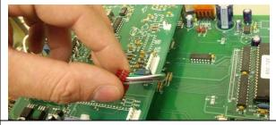
4. Remove the 3 screws securing the SCPC receiver to the standoffs.
