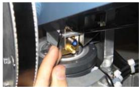
6. In order to pull out the drag link bracket first put an 11/32" open ended wrench over the nut and remove the screw from the other side of the yoke using a #1 Phillips screwdriver.
