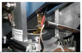
5. Remove the spacers attached to the bracket on both sides, put a 1/4" open ended wrench over the nut and remove the screws from the other side using a #1 Phillips screwdriver.
