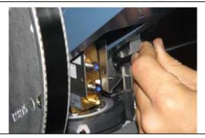
7. Pull out the drag link bracket; it is ok to bend the bracket a little if necessary. Be careful not to damage the power ring cables.
