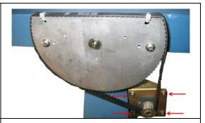
3. Apply Loctite 638 to the shaft of the replacement motor and fit the pulley in the same position as the one on the defective motor. Fit the set screws into the pulley with Loctite 222 using a 1/16" Allen wrench.
