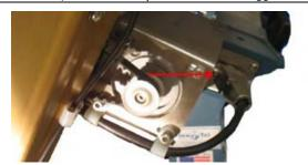
2. Using a 5/32" Allen wrench, remove the four Allen head screws attaching elevation motor bracket to CL beam and remove the motor assembly.
