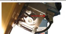
2. Using a 5/32" Allen wrench, remove the four Allen head screws attaching elevation motor bracket to CL beam and remove motor assembly.
