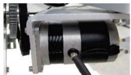
9. Align the bracket to beam and install the second bracket mounting screw and tighten both screws.
