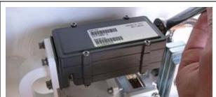
2. Using a 3mm Allen wrench undo the hardware securing the LNB to the waveguide and remove the LNB. Save the hardware for future use.
