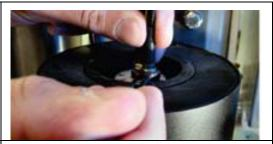
2. Using a 5/32" Allen head wrench, remove the four M4 screws that secure the Power Ring Assembly to the Adapter Plate. Retain hardware for future use.
