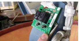
5. Apply Loctite 242 to both the screws and tighten them using a #1 Phillips screwdriver.
