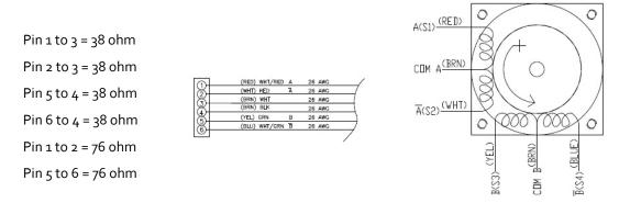
If one of the measuring points is open (no resistance) the motor is defective and needs to be replaced. Also measure from all the pins to ground (the metal case of the motor) they must be open, not shorted.
