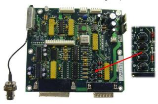
Set your multi-meter to the Diode setting and test between the pins of the transistors as per the following procedure and verify the results.
