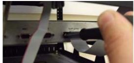
g. Using a #2 Phillips screwdriver remove the four screws securing the DAC to the front of the rack. Save the hardware for future use.
