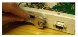
5. Using a 3/16" wrench or socket undo the jack screws from the D-sub connectors in the rear panel of the DAC and set aside.
