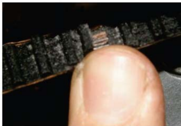
Separating tooth and edge wear
