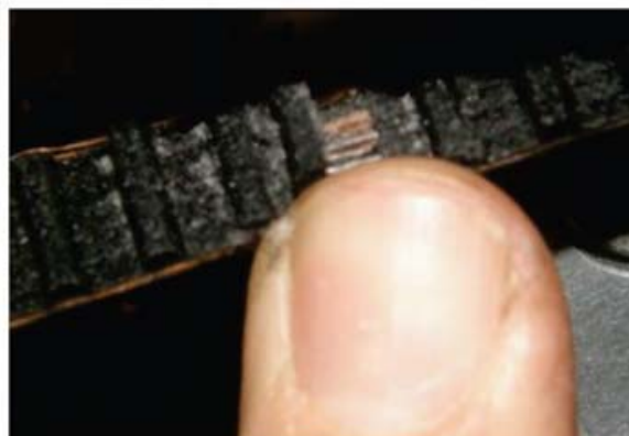
Seperating tooth and edge wear
