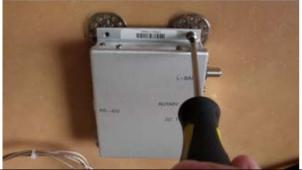
4. Install the replacement modem using the screws removed in the previous step and apply Loctite 242 to the threads. Then connect the interface harness & coax cable.
