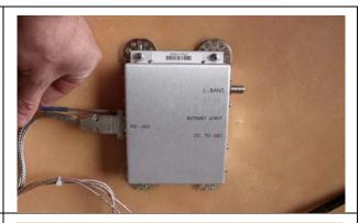
3. Using a #1 Phillips screwdriver, remove the 4 screws securing the modem into the radome base & save for future use.
