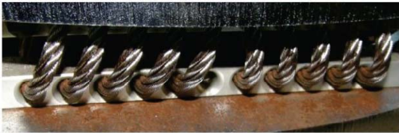
Rust from wire rope
