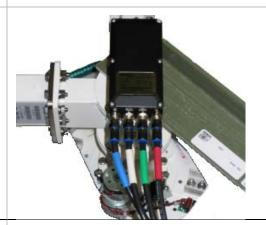
Loosen the Allen set screws on the existing LNB mounting collar (three set screws, 120 degrees apart) and remove it from the mounting collar.
